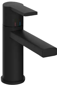
Walton Tall Mono Basin Tap 54w x 151d x 147h Min pressure - 1.0 bar - Reach 117.5mm
