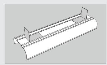
The profile should be secured to the carcass with supplied brackets which slot into the rear of the profile
