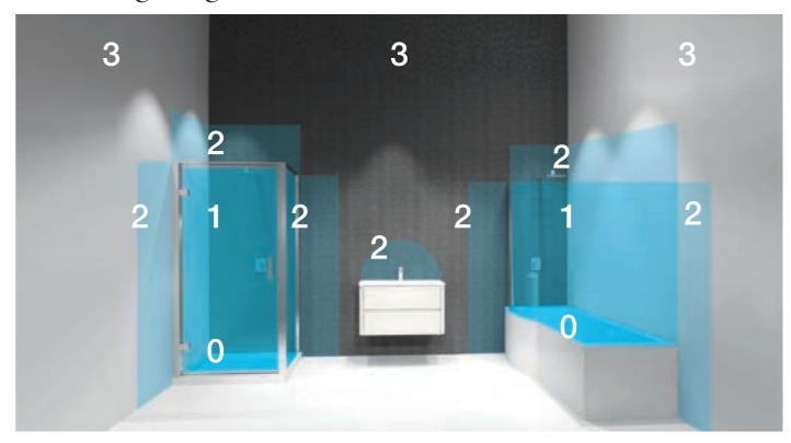
Water and electricity are a dangerous combination so when choosing bathroom lights it is essential that you familiarise yourself with two terms; Bathroom Zones and IP Ratings. When purchasing bathroom lights you need to ensure that the fitting you choose has the relevant IP rating for the zone in which it is to be placed. So what are IP Ratings and Bathroom Zones?
