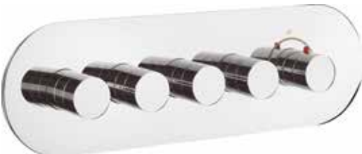
Thermostatic shower valve 4 control CE4001RC £899.00 Landscape Recessed Water pressure: HP3 4 independent flow controls with single temperature control See pages 292-303 for operation
