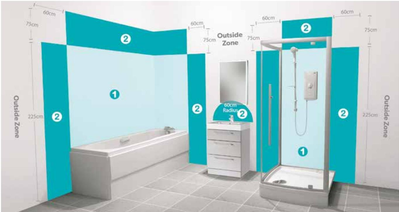
**Zone 1** refers to the area above the shower up to a height of 2.25 metres and requires a minimum rating of IP44 or higher and if the fitting is 240V a 30ma RCD must be used to protect the circuit.
