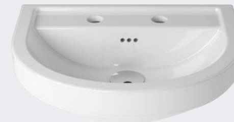
Monet Round semi-recessed short projection washbasin with integrated overflow and two tap holes, for use with a reduced-depth fitted washbasin unit
